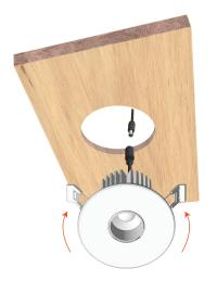
Connect the lead wire with jack from the light to the power source before inserting it into the routed/cut hole. While inserting the fixture, keep the spring clips held in the upward position..
