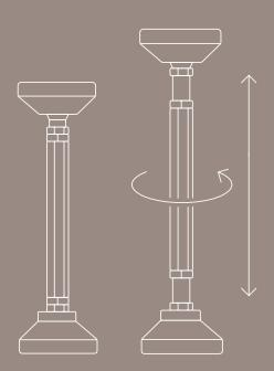
Extendable inner cylinder tightly secures mini fridge in cabinet
